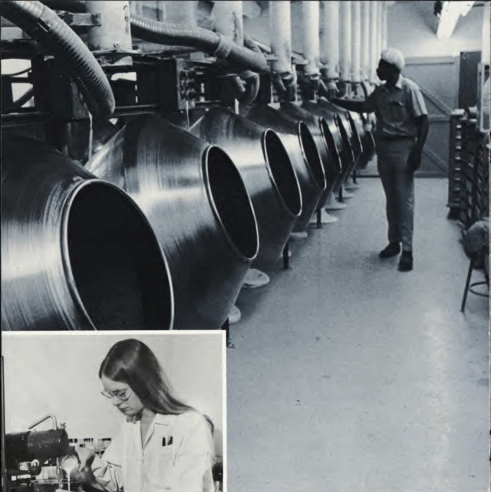
Above: Battery of tablet-coating machines in Chicago laboratory, under trained eye of Coating Specialist James E. Blue.
